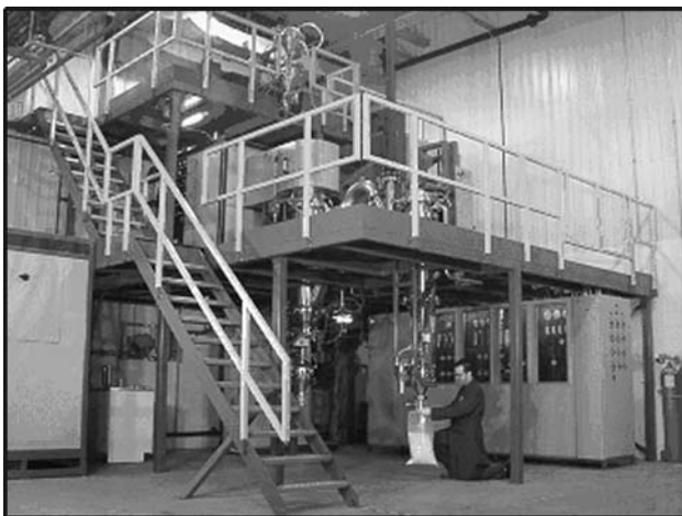
Fig. 8 Picture of an industrial set-up of 400 kW for powder spheroidization at Teckna (Ref 61)
